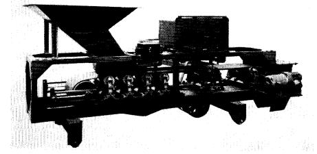
Portable Transportofeeder, a self contained automatic, feed regulating weigher,
